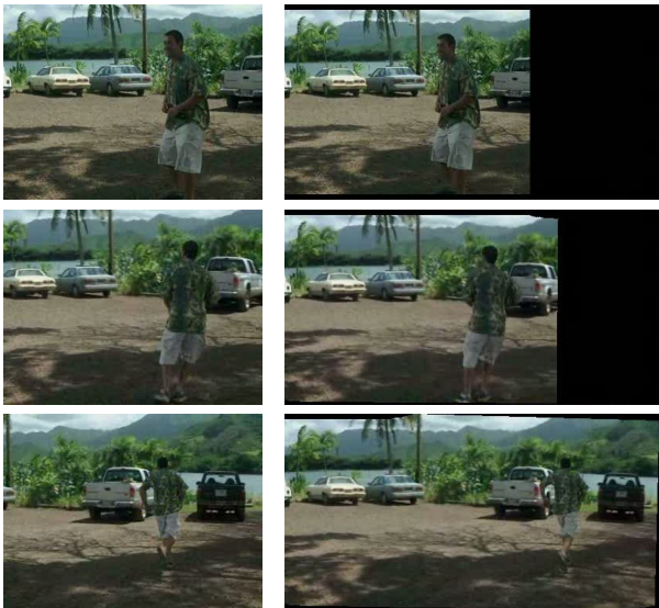
Figure 3. Examples of a clip stabilized over 50 frames showing from the top to the bottom, the 1st, 30th and 50th frame of the original (left column) and stabilized clip (right column).
